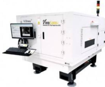
V810 S2EXi can handle boards up to 19" x 24" which is 10 percent larger than its predecessor – the V810 S2 system. It supports boards up to 7mm thick and 4.5kgs. With the introduction of the Motorized X-Ray Tube and Motorized Filter Height Sensor (FHS), V810 S2EXi offers greater top clearance up to 50mm and bottom clearance up to 70mm. High accuracy and repeatability are achieved with this motorized close-loop design.
