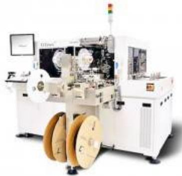
TR2000i's 14 pick-up nozzles enable machine throughput of up to 33K. Dual taper enables two running modes on the same device with 0 time reel change or different devices with 0 time taper conversion. Tri-nozzles pick & place allows faster unit pick-up for higher throughput of up to 18K (tray-to-tape). The three output stack/ tray has one good and two reject trays stacked for multiple binning. The second output track allows auto/ manual unloading to cater for different operation modes.
