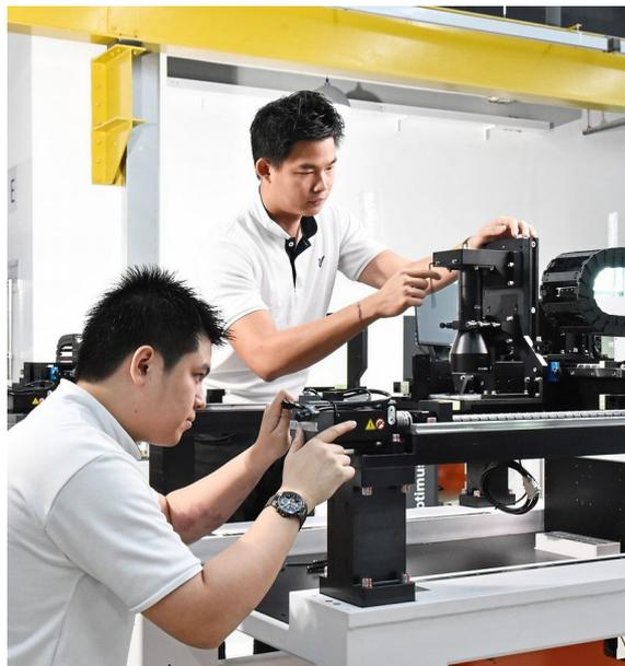
Manufacturing engineers assemble and conduct testing of the automated optical inspection system.
